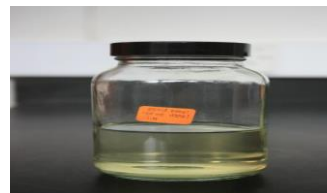
Figure:26 60 ml of emulsifier and 10.92% of hydrogen peroxide with pure diesel
