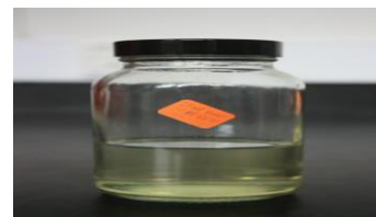
Figure:24 20 ml of emulsifier and 3.50% of hydrogen peroxide with the pure diesel
