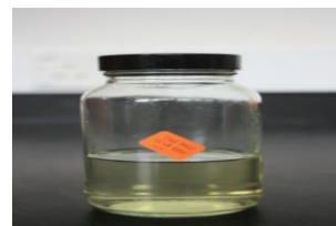
Figure:23 10 ml of emulsifier and 2.53% of hydrogen peroxide with the pure diesel
