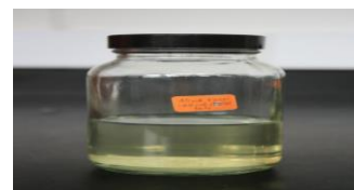
Figure:25 40ml of emulsifier and 6.34% of hydrogen peroxide with the pure diesel
